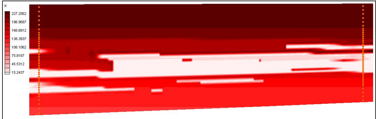
Figure 4.7: Cross-Section View of Permeability Distribution (deep red color indicates high permeability and white color indicates low permeability area).
