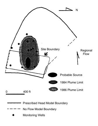
Figure 4-21. Extent of TCE plume in 1984 and 1986; also shown is the ground-water model domain, with prescribed (fixed) head and no-flow boundaries (34).
