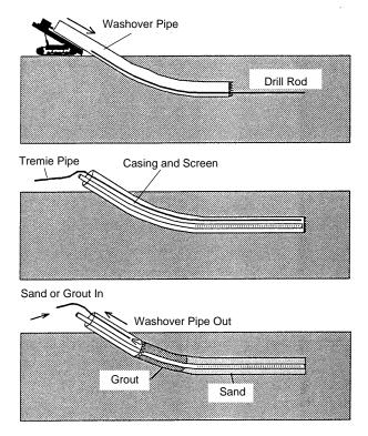
Figure 2-9. Completing a blind well using the washover pipe method.
