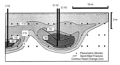
Figure 3-21. Cross section along line of piezometers showing change in head after 5 days of pumping.
