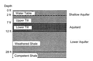
Figure 4-19. Typical subsurface profile (34).
