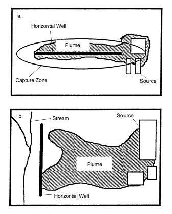
Figure 2-18. Two approaches using horizontal wells to intercept contaminant plumes.
