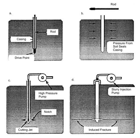
Figure. 3-6. Fractures created at the bottom of driven casing.
