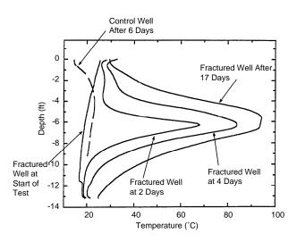
Figure 3-17. Temperature as a function of depth and time.
