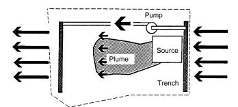
Figure 4-10. Controlling the flow through a contaminated area by pumping from an upgradient trench and injecting into a downgradient trench.
