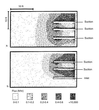
Figure 3-14. Flux of air to three flat-lying fractures (white band) shown in cross section: a) suction of 100 inches of water on all three fractures, and b) air inlet (atmosheric pressure) at the bottom and suction on the other two fractures.
