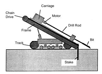
Figure 2-3. Directional drilling rig.
