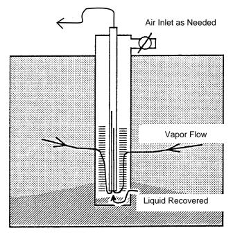
Figure 3-15. Well configuration to recover liquid and vapor phases using suction at the ground surface.
