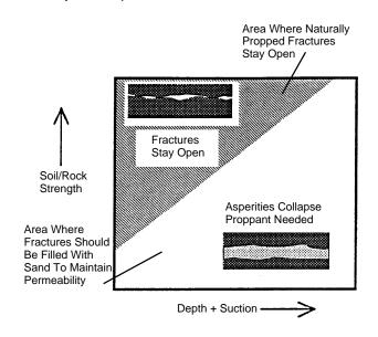
Figure 3-13. Factors that affect how fractures should be propped.
