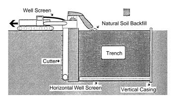
Figure 4-2. Schematic of continuous excavation and completion technique (6).
