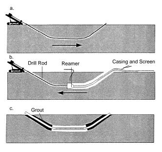
Figure 2-8. Creating a horizontal well with the pull-back method: a) drilling a continuous wellbore, b) reaming and pulling in casing, c) the finished well.
