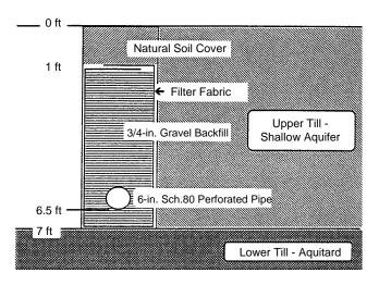
Figure 4-25. Schematic cross section of trench construction (38).
