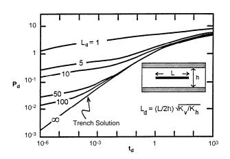
Figure 2-15. Drawdown resulting from a horizontal well as a function of time and dimensionless length. Drawdown and time are dimensionless.
