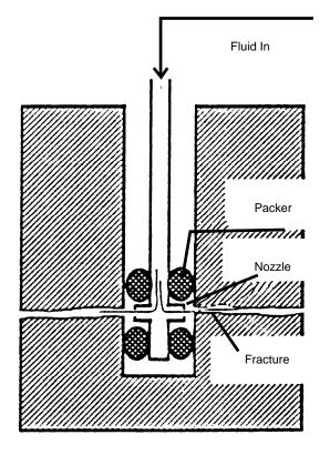
Figure 3-5. Fracture created by isolating a zone with a straddle packer.
