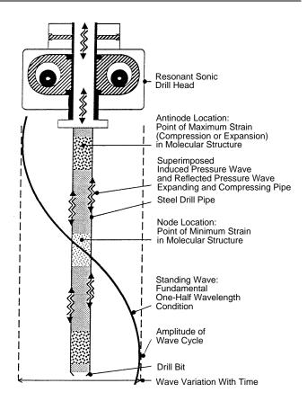
Figure 2-6. Resonant stress wave providing energy to the drill bit (10).
