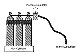
Figure 3-4. Aboveground equipment used for pneumatic fracturing (9).
