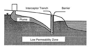
Figure 4-11. Interceptor trench coupled with a hydraulic barrier to minimize recharge from an adjacent surface waterbody.
