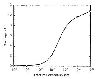
Figure 3-8. Air discharge from a well intersecting a flat-lying circular fracture as a function of the permeability of the fracture. (Formation permeability is 10<sup>-9</sup> cm<sup>2</sup>.)
