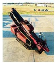
Horizontal directional drilling has been used for the installation of wells for a number of different environmental applications. Courtesy of Advanced Directional Drilling Systems.
