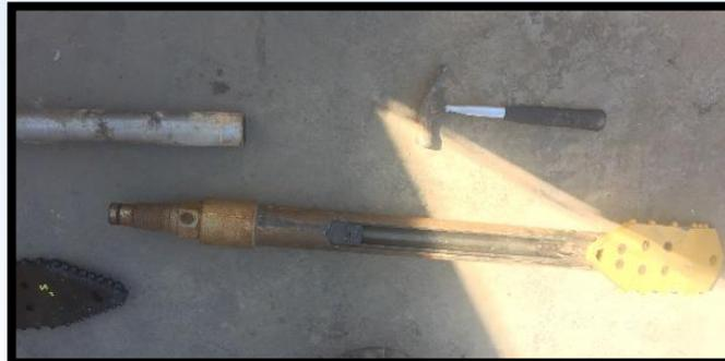
*Drill bit housing with sonde*
