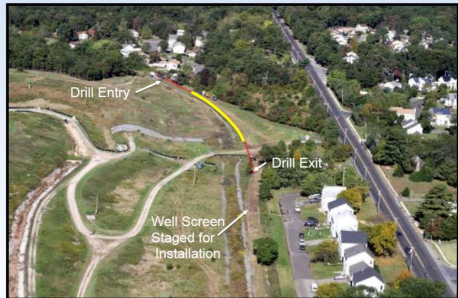
*Horizontal Hydraulic Control Well for Landfill Leachate Containment*
