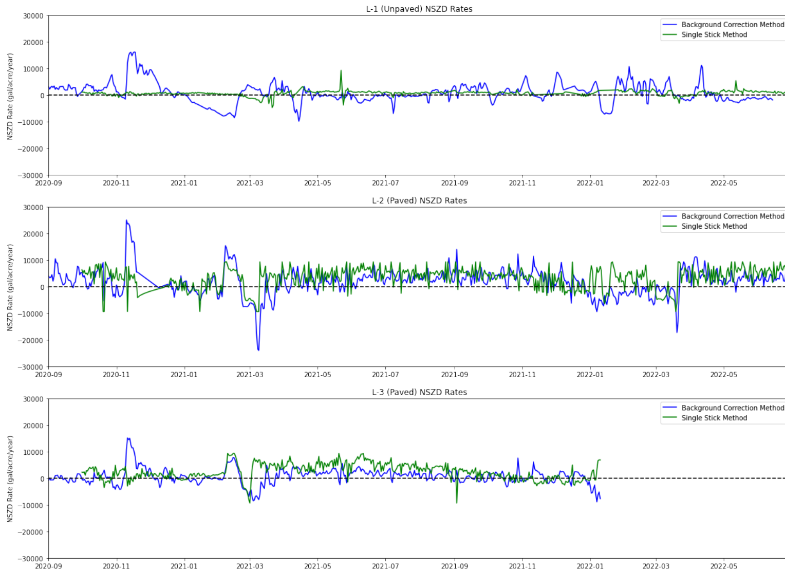
Figure 6.6. Comparison of Method 2 Background Corrected Method and Method 3 Single Stick Method Over Time at the MN ANGB.
