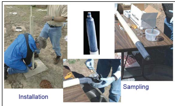
Photo of installation of passive flux meter (above). How flux meter works (right). (Photos courtesy of Enviroflux).
