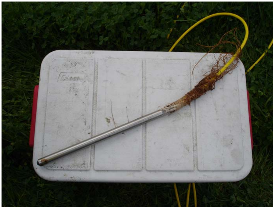
Photograph taken February 2005 at monitoring well 755PHYTO25, which contains an In-Situ ® pressure transducer. This shows the roots that were pulled up when the sensor was removed from the well. The roots consisted of tough/woody red roots at the top (above the water table) and wet/smooth white roots that were in the groundwater.
