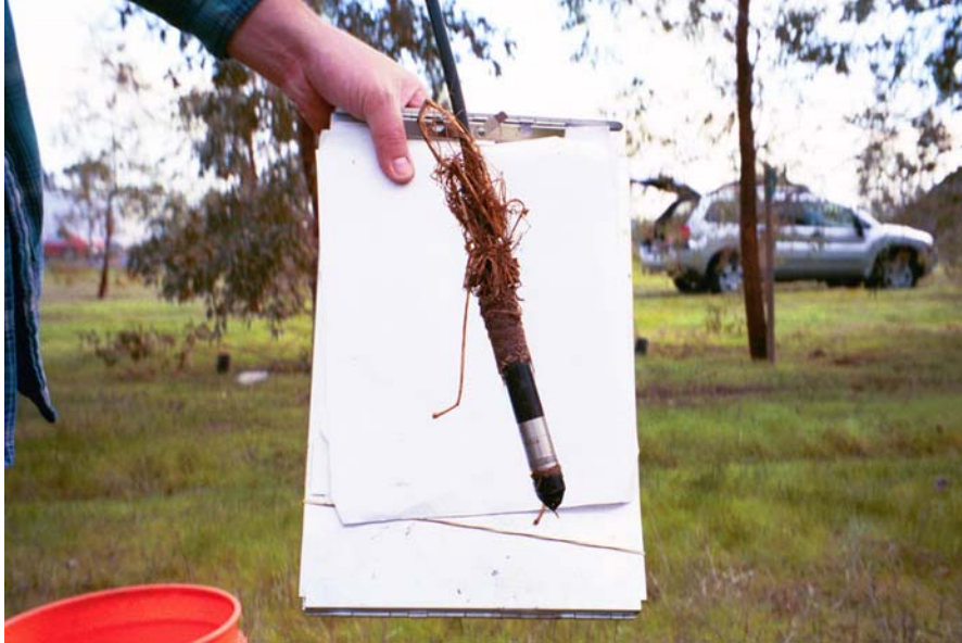
Photograph taken February 2004 at monitoring well 755PHYTO32, which contains a Druck ® pressure transducer. This shows the roots that were pulled up when the sensor was removed from the well.
