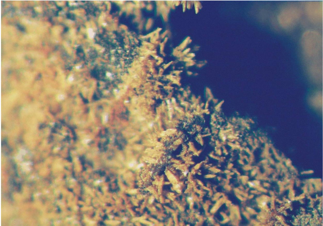
Figure 17. Photomicrograph image of bladed calcium carbonate crystals nearly completely coating the surface of a ZVI grain. Sampled October 28, 2004, 1 ft above base of ZVI and 0.5 ft from upgradient face of ZVI. Width of photo 2 mm.
