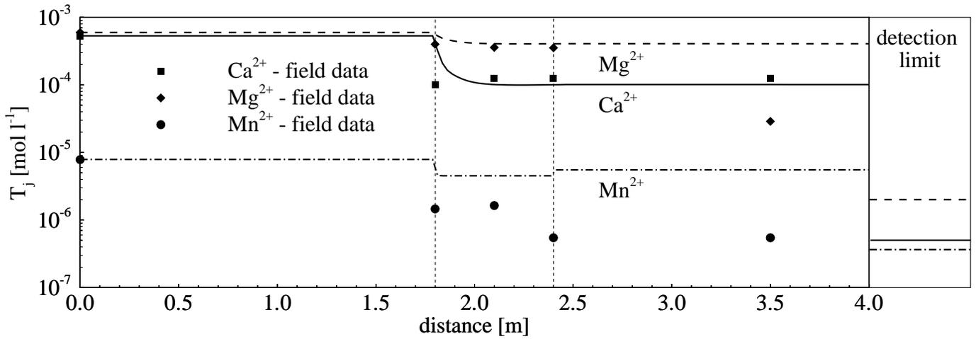
Figure 9. Selected cation concentrations after  $t = 240$  days - one-dimensional simulation.
