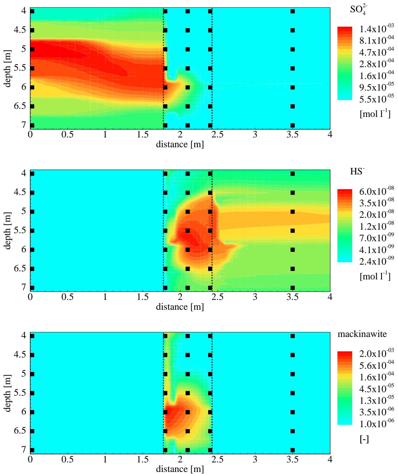
Figure 18. Sulfate and sulfide concentrations and mackinawite volume fractions after  $t = 2$  years.
