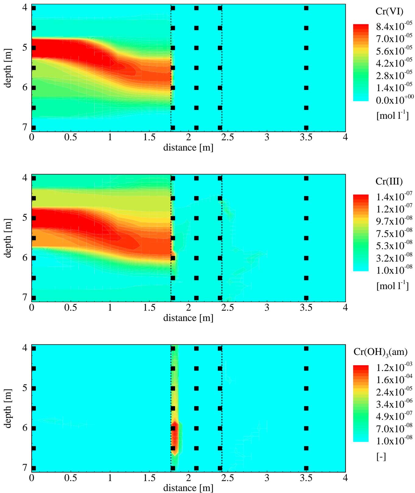
Figure 15. Hexavalent and trivalent chromium concentrations and Cr(OH)<sub>3</sub>(am) volume fractions after t = 2 years.
