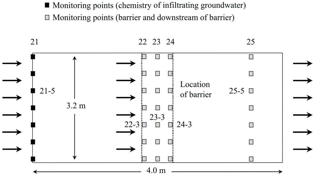
**Figure 4.** Solution domain including location of barrier and monitoring points along Transect 2.
