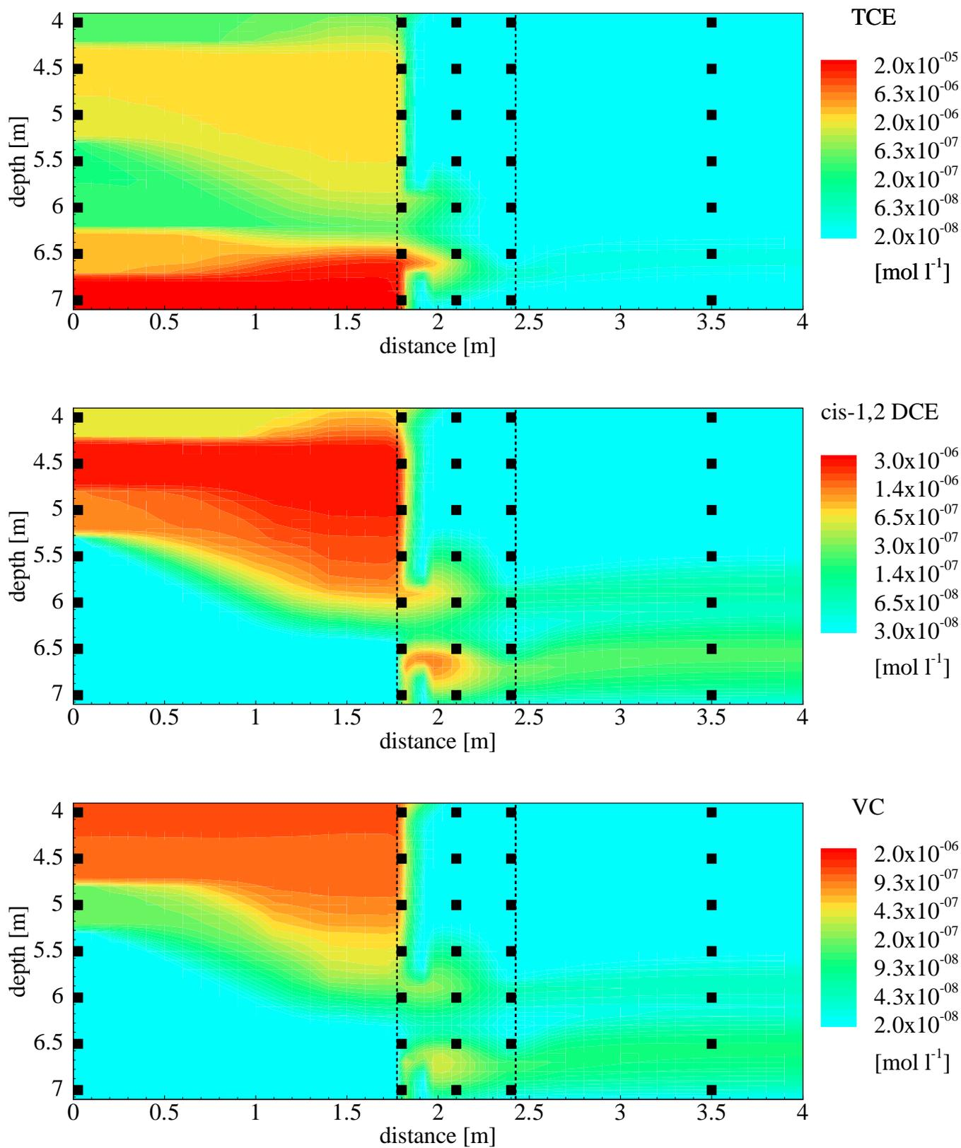
Figure 16. TCE, cis-1,2 DCE and VC concentrations after  $t = 2$  years.
