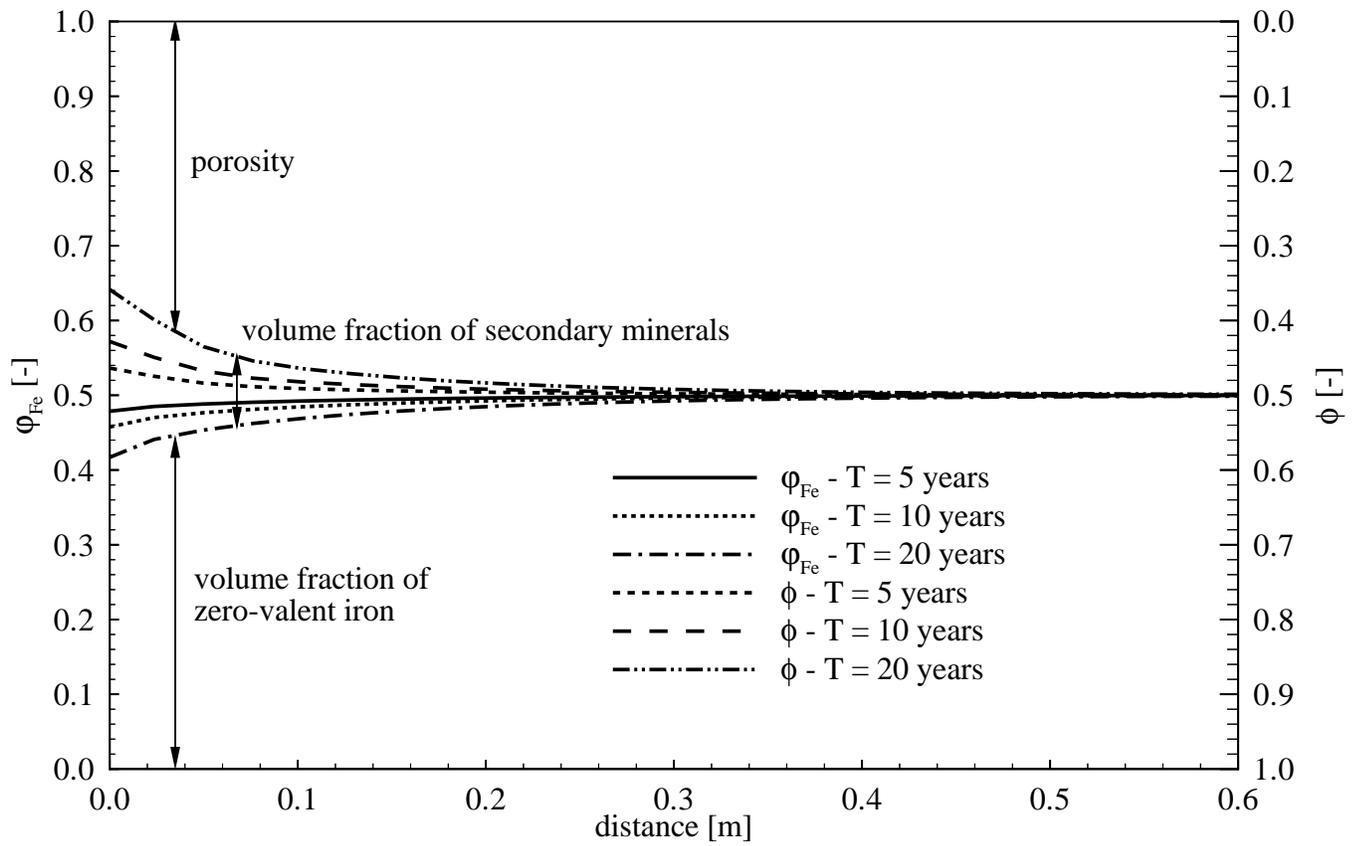
Figure 13. Long term effect of iron corrosion and secondary mineral formation.
