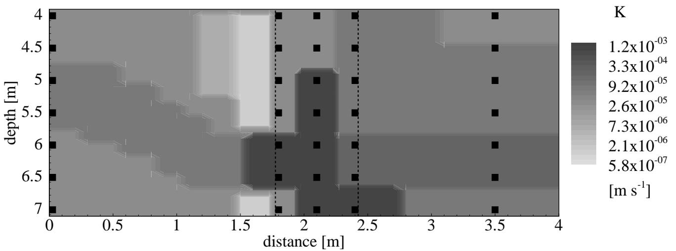
Figure 6. Hydraulic conductivity distribution in two-dimensional solution domain, modified from Bennett [1997].
