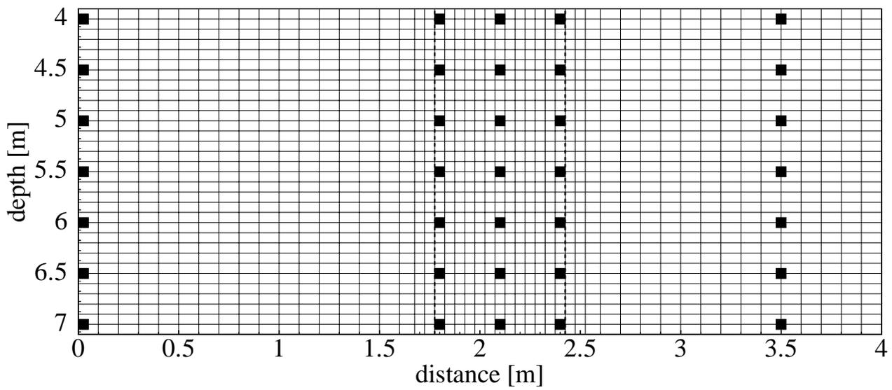
Figure 5. Spatial discretization of two-dimensional solution domain.
