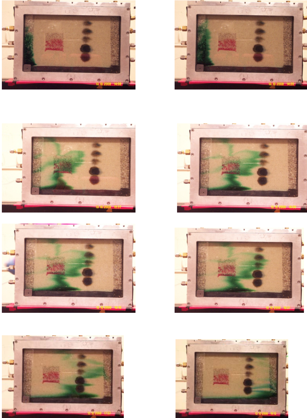
Figure 7.6.10. Selected photos illustrating the flow pattern when a food dye was used as a tracer.
