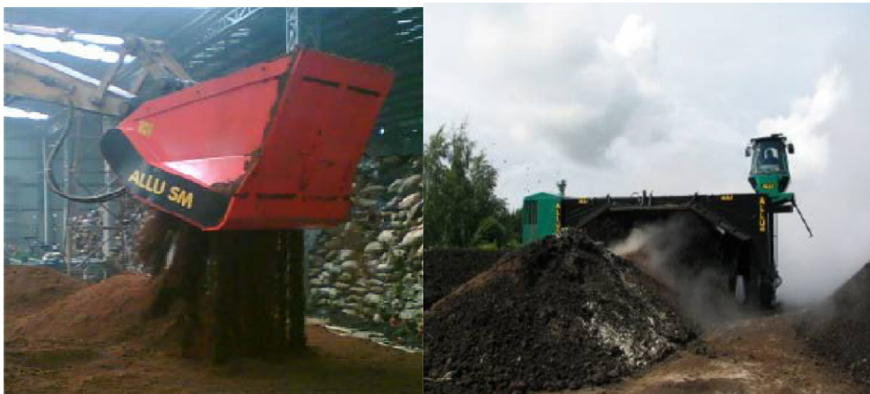
Figure 7. Pictures show STSO mixing equipment of binders and material. Left fig: Screen crusher, right fig: Window turner (Lasse Lintermo, Allu Finland OY).
