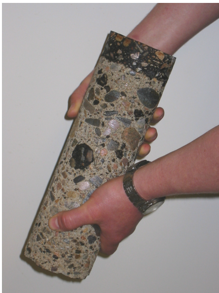
Figure 27: A follow-up sample from a layer-stabilized road in Rautavaara in the autumn 2005. The project was carried out in the summer 2004. Here, the existing asphalt pavement was crushed and mixed into a depth of 200 – 300 mm with the binder (a composite of cement and fly ash). After stabilization a new pavement was spread on the surface. (Ramboll Finland Oy)
