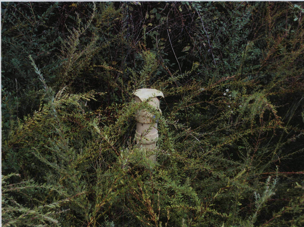
Photo 15: Well MW-29, overgrown.
