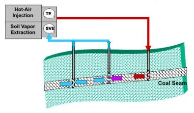
Step 3: Soil Vapor Enhanced with Hot-Air Injection - Relay to Second Injection Row
