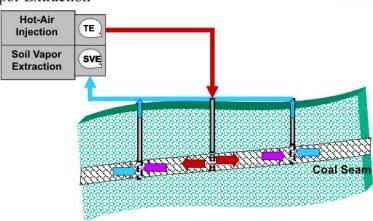
Step 2: Soil Vapor Enhanced with Hot-Air Injection – Initial Injection Row
