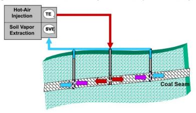
Figure 1. Thermally enhanced SVE – well field relay.
