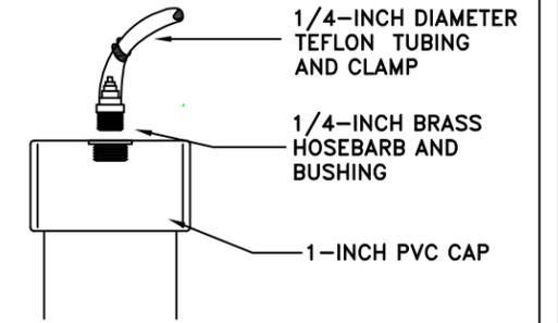
TYPICAL BELOW GRADE VAPOR PROBE DETAIL
