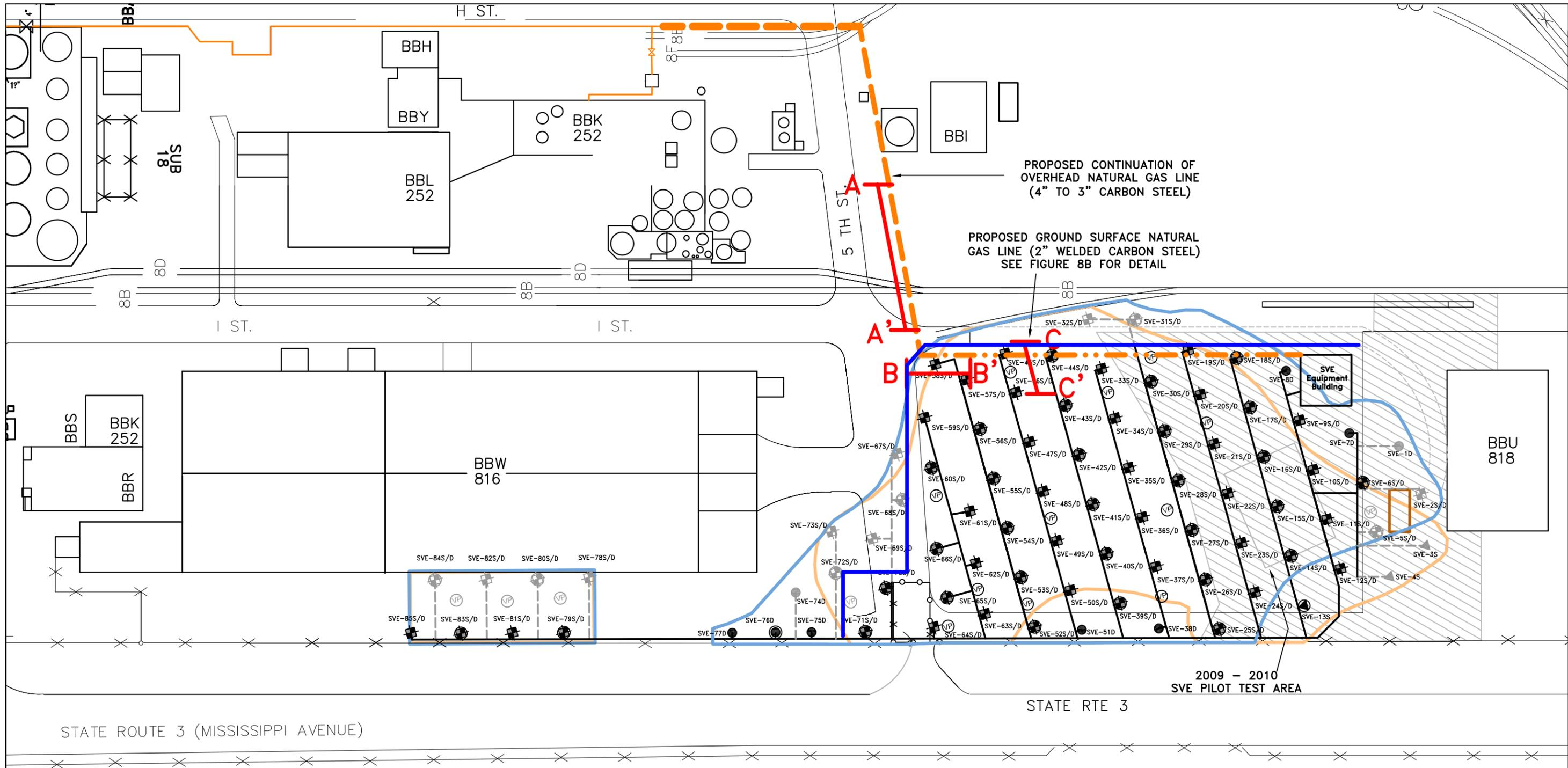
PROPOSED CONTINUATION OF OVERHEAD NATURAL GAS LINE (4" TO 3" CARBON STEEL)
