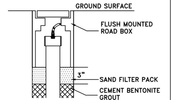
TYPICAL BELOW GRADE SVE/AI WELL COMPLETION DETAIL
