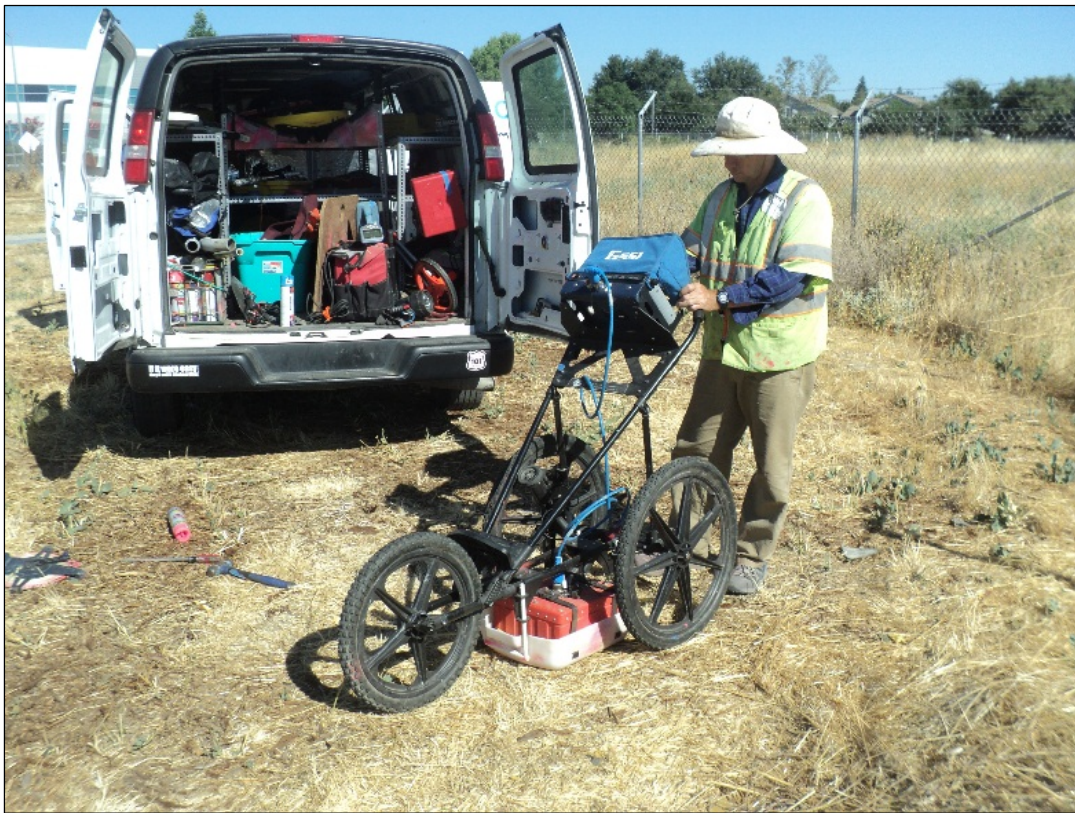
Ground-penetrating radar performed to search for additional voids.
