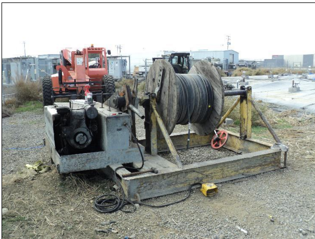
Wire rolling equipment.
