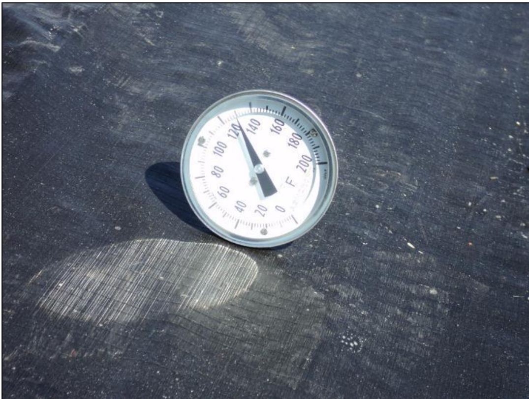
Temperature on the cap at 16:50 was near 130 degrees Fahrenheit.
