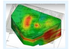
High-resolution, three-dimensional imagery helps guide bioremediation implementation at the Bay Road Holdings LLC (formerly Romic) site in East Palo Alto, California. The project involves injections of amendments providing a food source for naturally occurring microorganisms capable of degrading contaminants in an angerobic environment.
