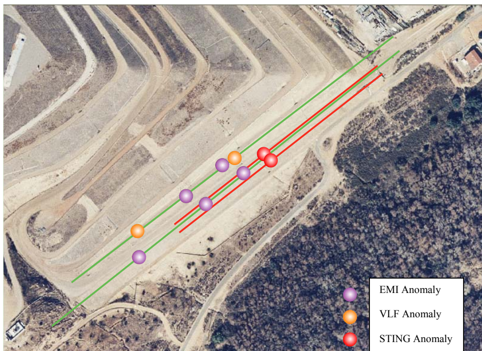
Figure 2 - EMI surveys identified anomalies oriented N85°W which correlate to high-angle joints in outcrops west of the site. VLF surveys identified several anomalies with apparent orientations of N55°E.
