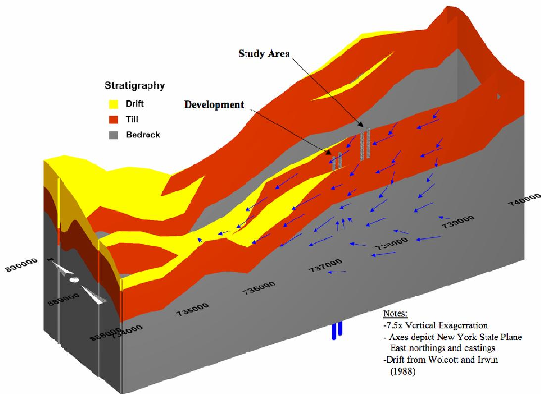
**Figure 6:** Suspected ground water flow within and between the bedrock and glacial aquifers.
