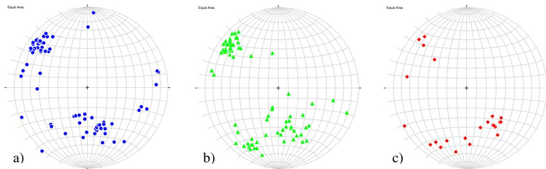
**Figure 5:** Lower hemisphere plots of poles to planes for planar features identified by ATV. The features are separated into three classes based on apparent aperture: Class I is depicted in (a), Class II in (b), and Class III in (c). Note the tight clustering of poles in (a) and (b) corresponding to planar features with northeastern strikes and south and east dips.
