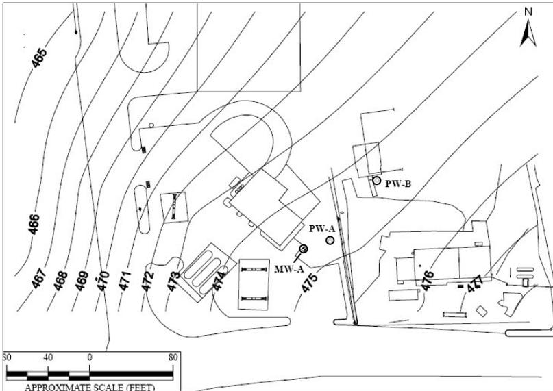
**Figure 1:** Site plan including the adjacent retail petroleum service stations and residence at the study area with water table elevation contours derived and inferred from 21 overburden wells not depicted.
