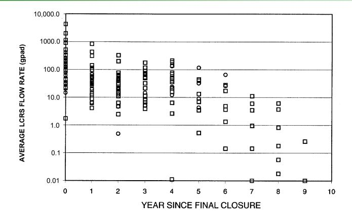
Average LCRS flow rates (lhd) after closure for eleven MSW cells (shown as circles)and 22 HSW cells (shown as
