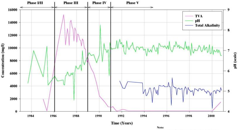
Phase designation references the phases of waste degradation presented in Figure 2, after Pohland and Harper, 1986.
