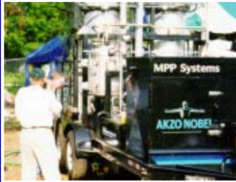
Trailer-mounted MPP system
